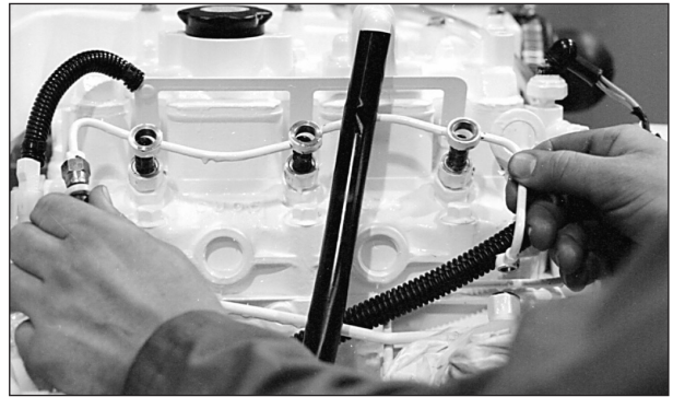
Figure 15: Remove return line.
