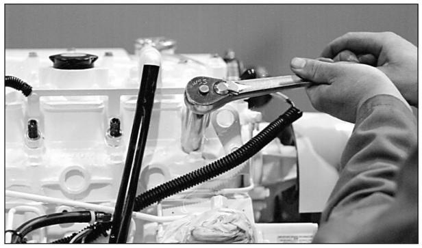
Figure 18: Reinstall injector. Torque to proper tightness.
