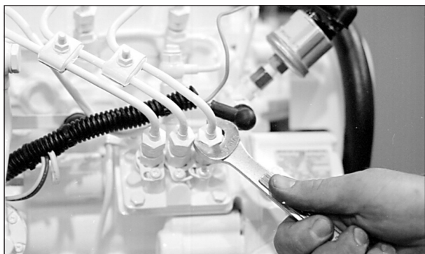
Figure 13: Remove delivery line flare nuts.
