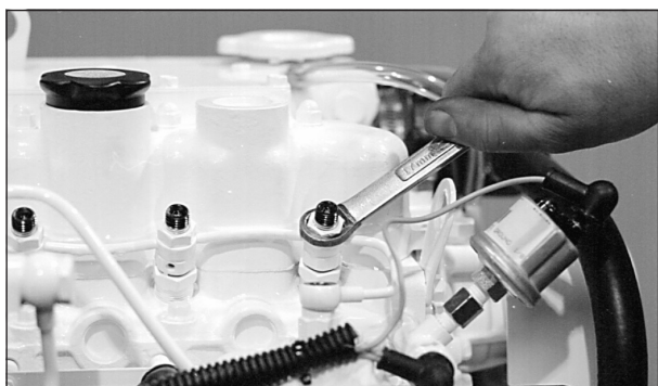
Figure 16: Remove return line nuts.
