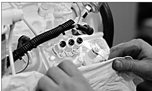
Figure 15: Cover lines, inlets and injection pump outlets.
