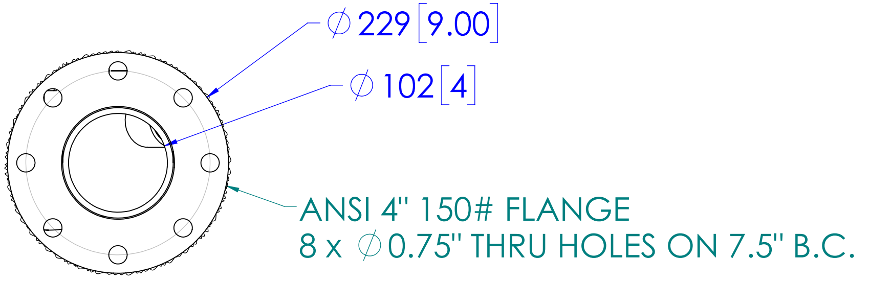
DETAIL A OPTIONAL DRY EXHAUST FLANGE SCALE 1 : 4
