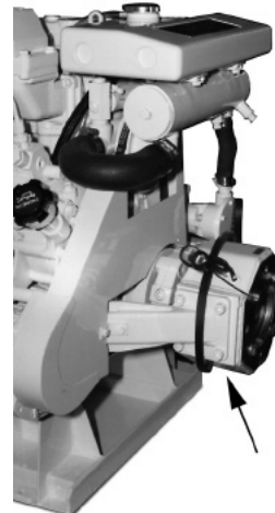
Figure 15: Optional PTO with electric clutch
