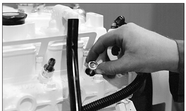
Figure 17: Remove and replace copper sealing washer.
