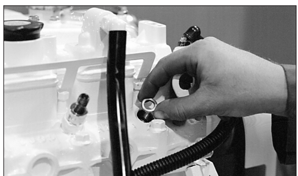
Figure 16: Remove and replace copper sealing washer.
