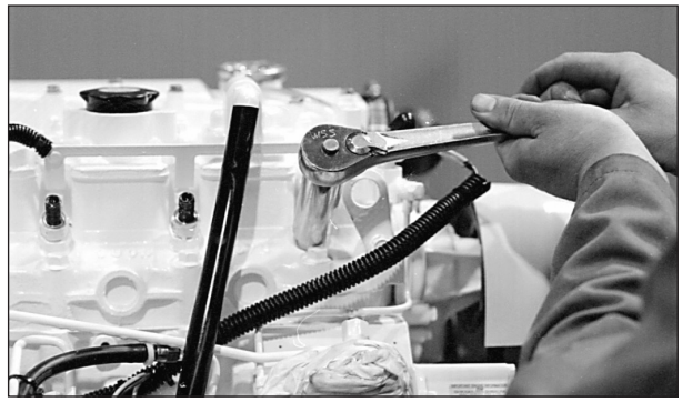
Figure 17: Reinstall injector. Torque to proper tightness.
