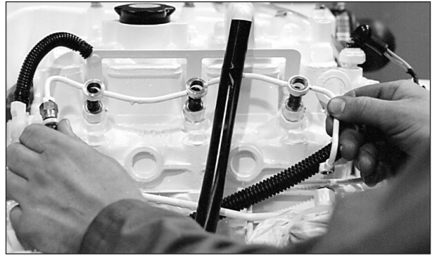
Figure 14: Remove return line.
