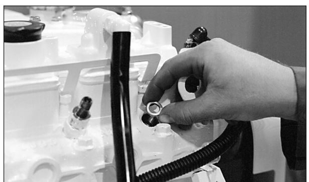
Figure 16: Remove and replace copper sealing washer.
