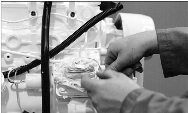
Figure 12: Cover lines, inlets and injection pump outlets.
