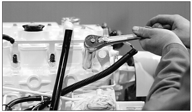
Figure 17: Reinstall injector. Torque to proper tightness.
