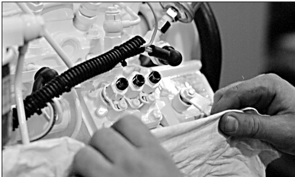
Figure 15: Cover lines, inlets and injection pump outlets.
