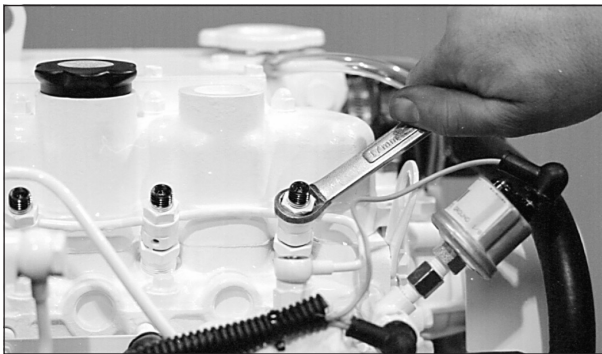
Figure 16: Remove return line nuts.
