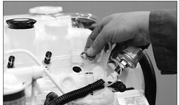
Figure 19: Remove and replace copper sealing washer.
