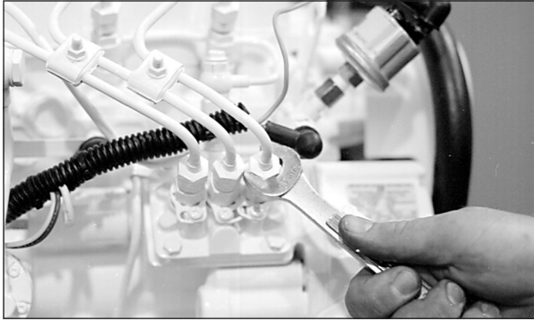
Figure 13: Remove delivery line flare nuts.
