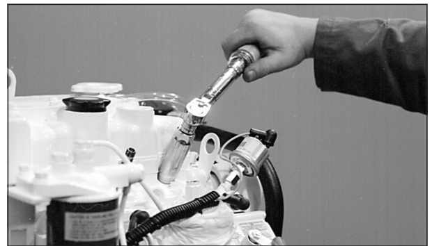
Figure 20: Reinstall injector. Torque to proper tightness.
